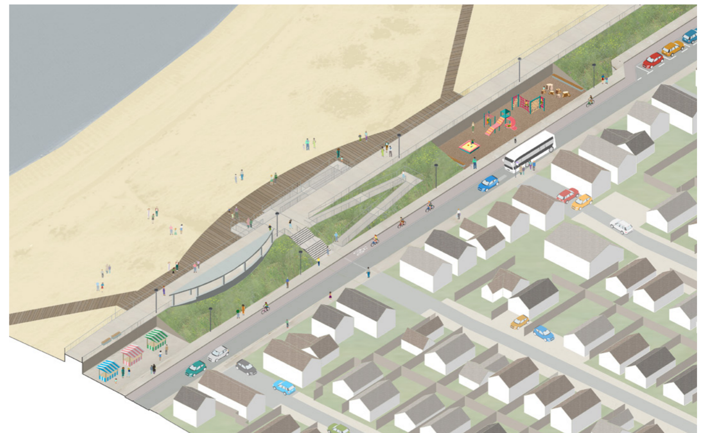
Fig. 5. Isometric sketch showing the main elements of the seafront design strategy along the Brooklands seafront
